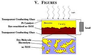
Figure 1: Schematic picture of the dye solar cell (on top) and its operating principle (below).
