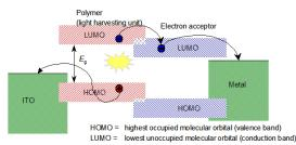
Figure 3: Schematic diagram shows the operation in organic solar cell
